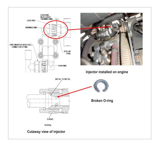
Sealing between the injector and the manifold is ensured by tightening, metal against metal, to a torque level defined by the manufacturer. The two O-rings create an additional safety when this tightening is not correct. Any damage to them can lead to a leak.
