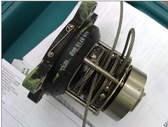
Loop formed by free part of cable that blocked the autopilot servo
