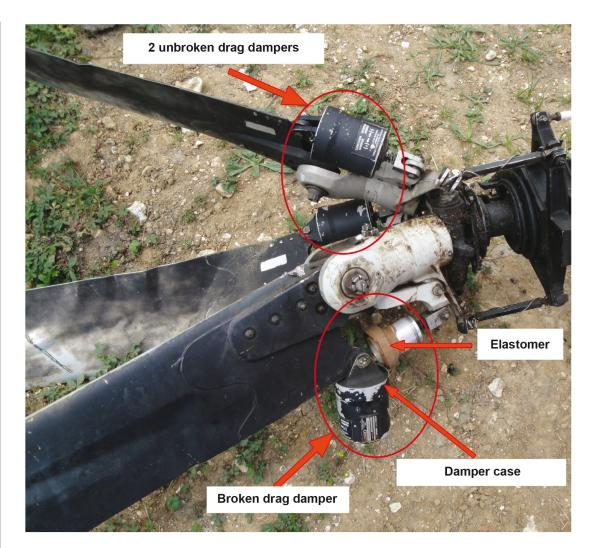
The technical examinations performed on the 3 drag dampers brought to light the following points:
