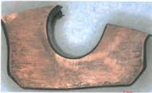
Fig. 42. Fragments of the diffuser aft seal analysed by LHT. Photo: LHT.
