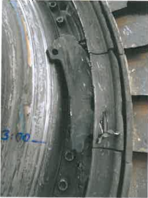
Fig. 57. HPT guide vanes stage one with fragments of the diffuser aft air seal. Photo: SHK.
