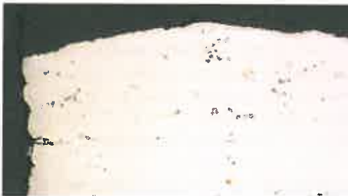
Fig. 43. Cross sections of the attachment lug with micro cracks, diffuser aft air seal. Photo: LHT.
