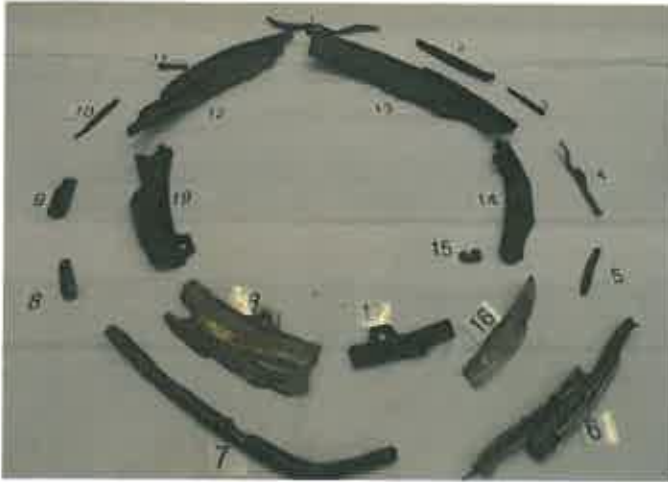
Fig. 42. Fragments of the diffuser aft seal analysed by LHT. Photo: LHT.
