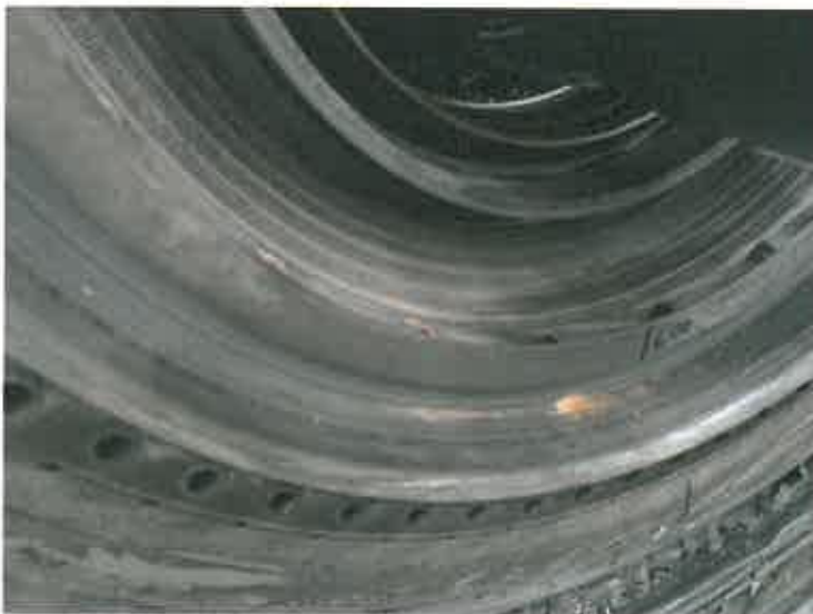
Fig. 37. Stationary seal, forward and aft (honeycomb completely torn away). Photo: SHK.
