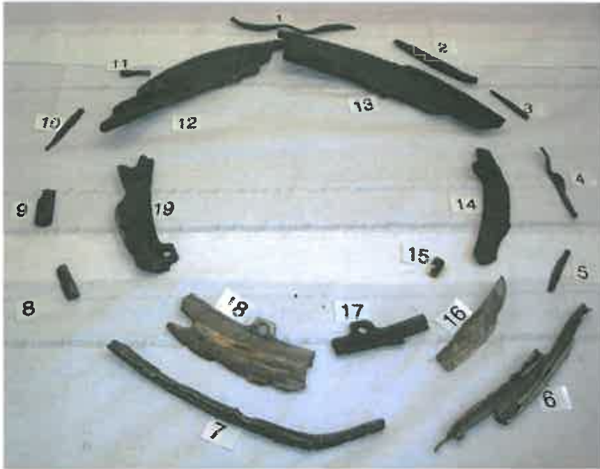
Photo No 2. LHT photo showing Diffuser Aft Seal fragments.
