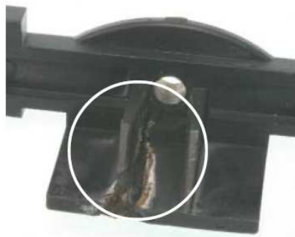
Unacceptable (Developing bearing bar failure)
