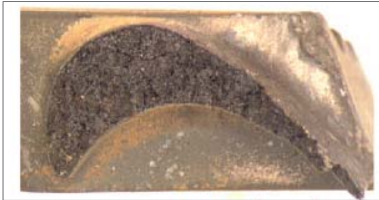
Photo n° 47 Typical condition of the CT blade fracture surfaces
