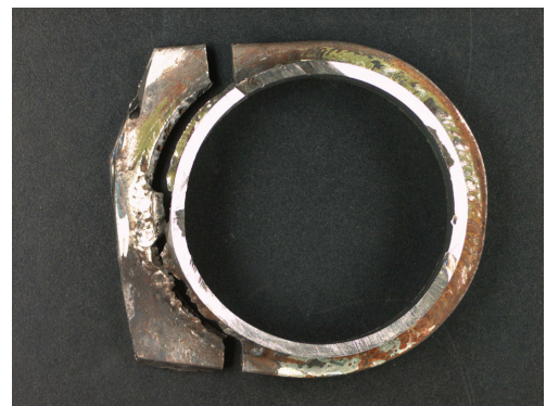
General view of failed weld seam (from below)
