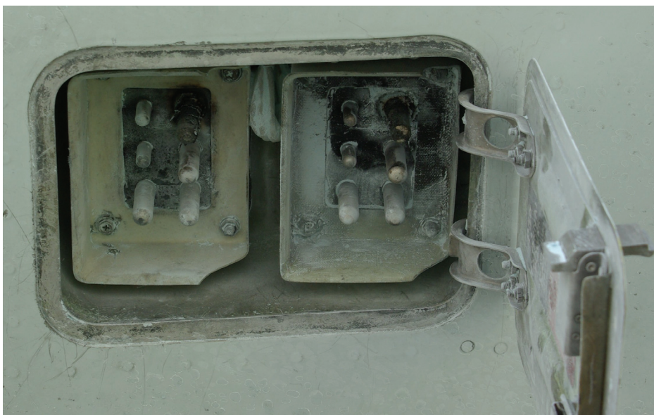
Electrical connectors from B-HOV a short time after the incident
