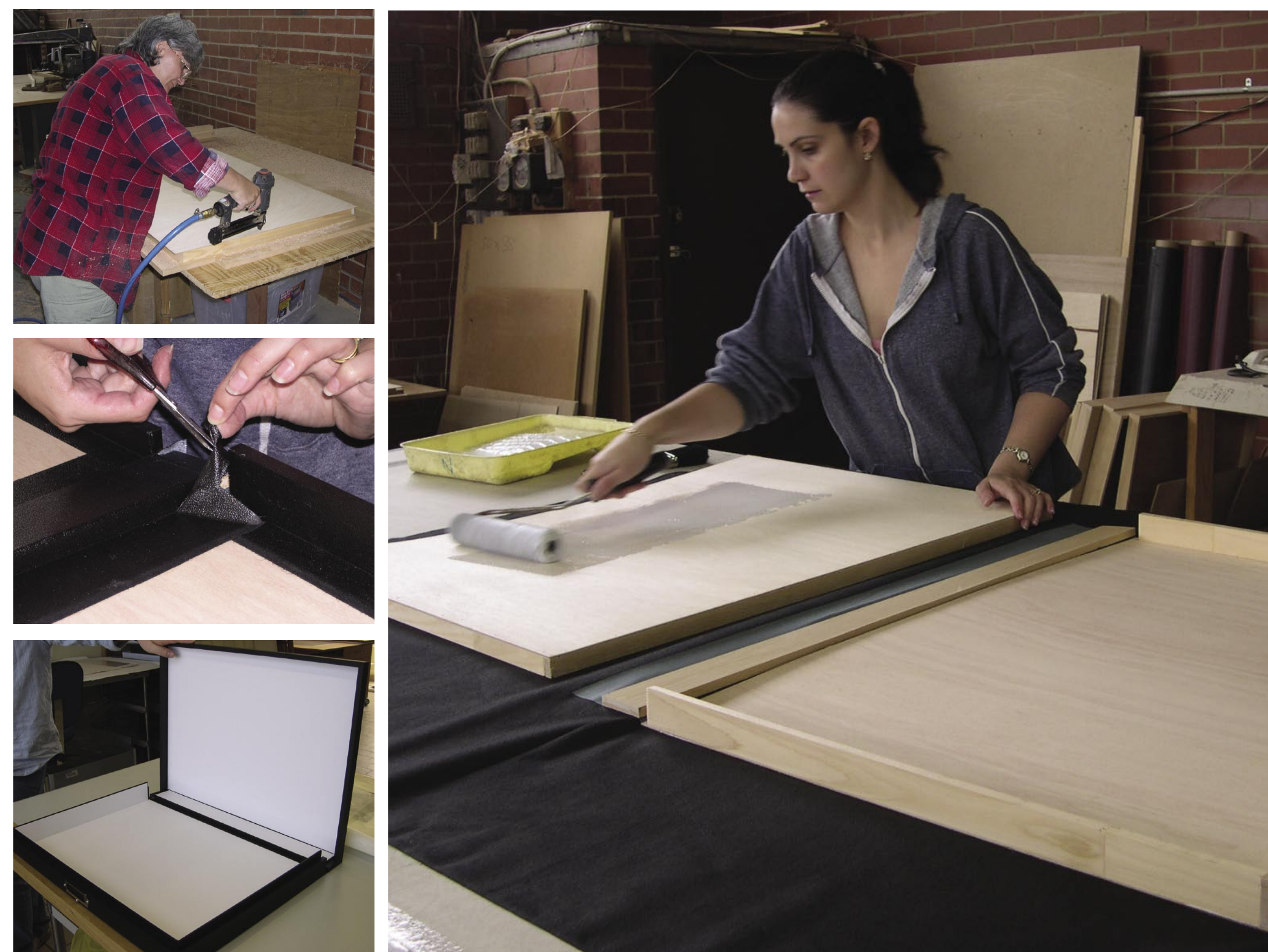
Stages in the construction of a National Gallery of Australia Solander box
