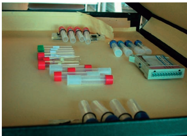
Figure 1 Box A: passive sampling experimental set-up.
