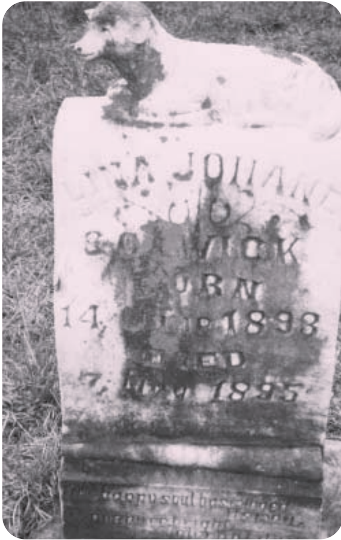
The woolly coat on the lamb adorning this infant's grave marker is disappearing bit by bit because of chemical weathering.
